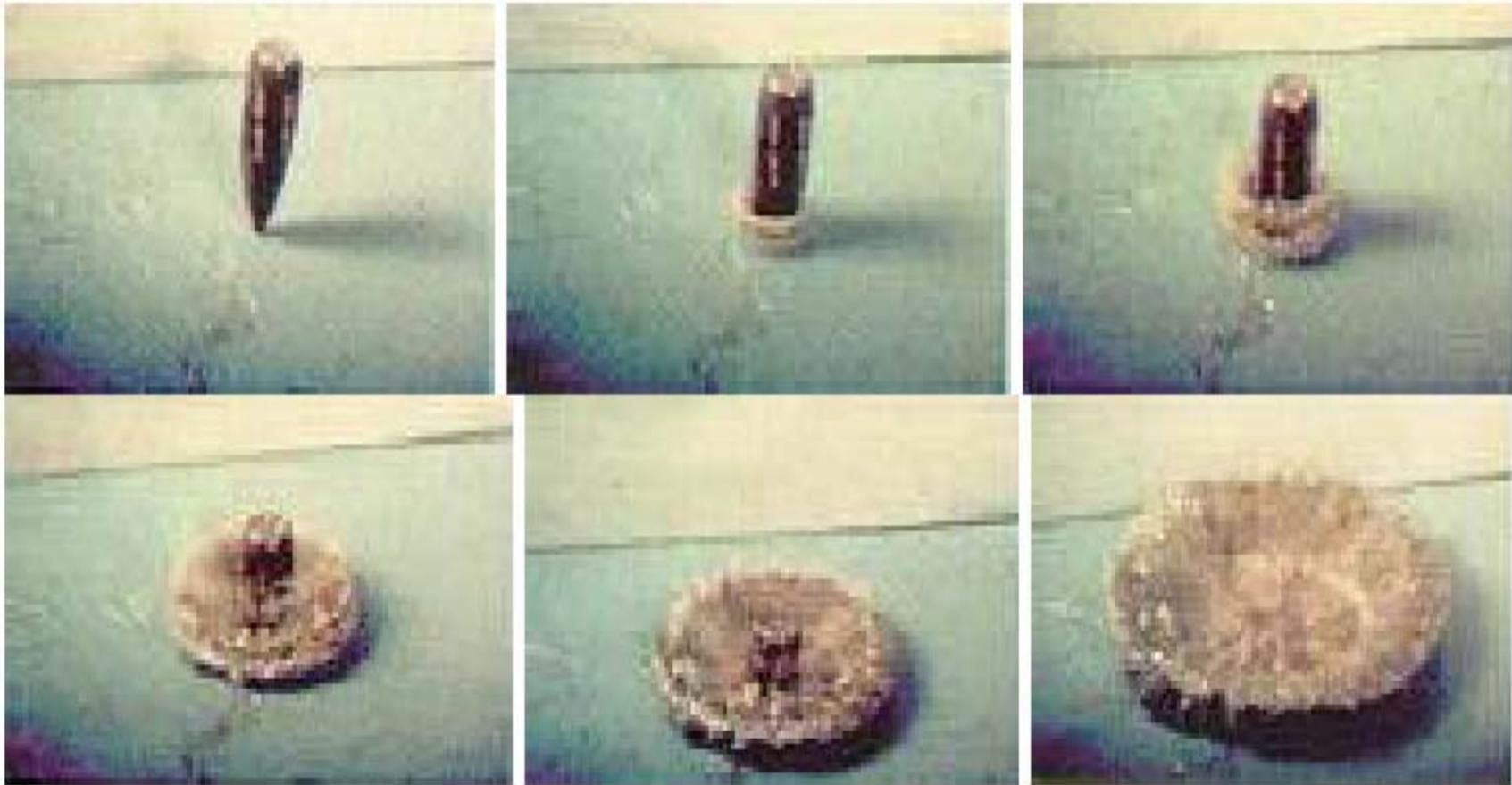
**.30 cal. bullet impacting hard steel at 2750 ft/sec**
