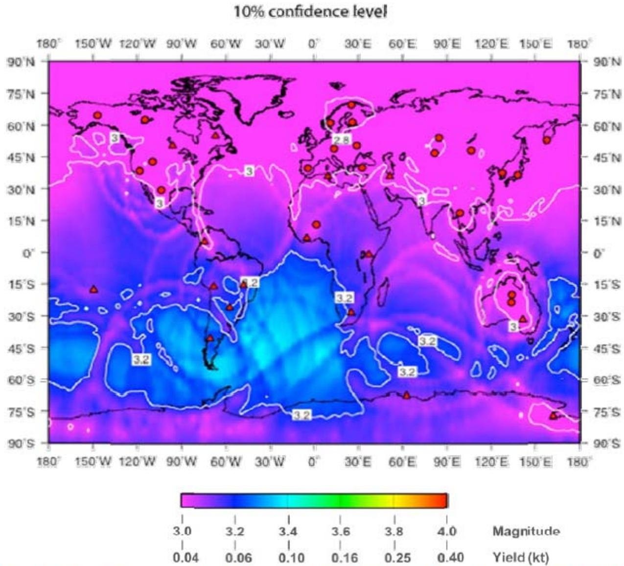
**FIGURE 4-1:** Map of 10 percent confidence detection levels (90 percent probability of avoiding detection) for the primary IMS Network (2007). The map represents detection capability of IMS primary seismic network, late 2007, with 38 stations sending data to the IDC. Contours indicate the magnitude of the smallest seismic event that would be detected with a 10 percent probability at three or more stations. Red circles are seismic arrays, and triangles are single seismic
