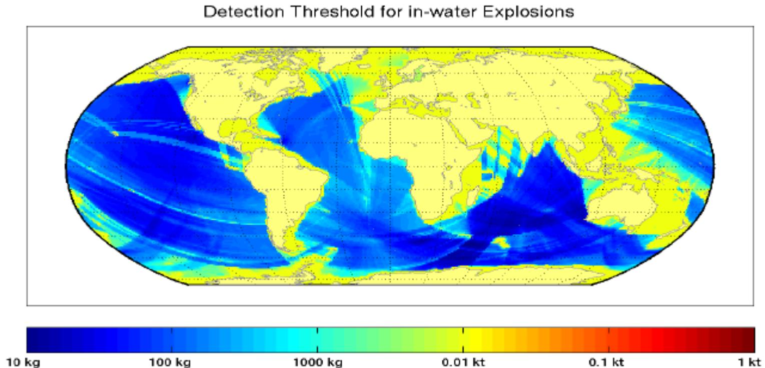
**FIGURE 2-11:** Map showing the IMS detection threshold in equivalent mass of TNT for in-water explosions detected on either the hydroacoustic or seismic IMS networks. Note that 1000 kg = 0.001 kt. Areas not covered by the hydroacoustic network—such as the Mediterranean Sea—are covered by the seismic network to a threshold of around 0.01 kt. SOURCE: CTBTO
