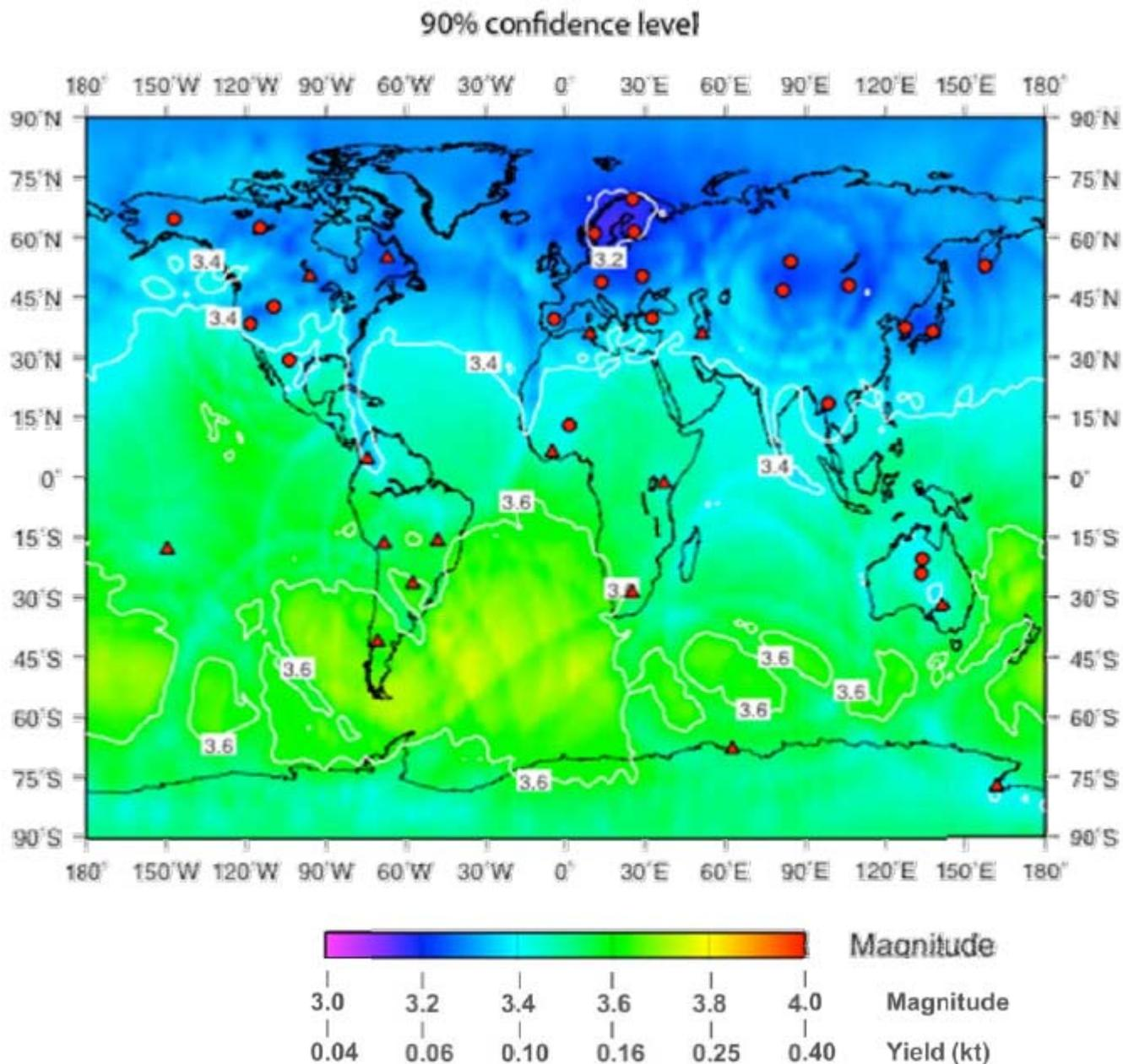
**FIGURE 2-8:** Detection Capability of the IMS Primary Seismic Network in late 2007, with 38 stations sending data to the IDC. Contours, indicate the magnitude of the smallest seismic event that would be detected with a 90 percent probability at three or more stations; that is, at enough stations to enable a location estimate. Red circles are seismic arrays, and triangles are
