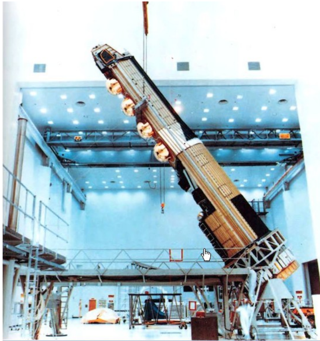
The HEXAGON photographic satellite vehicle. Length 60 ft; diameter 10 ft
