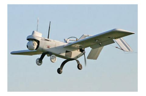
Bat 3 is a complete man-portable UAV system that operates autonomously from unimproved areas and delivers high quality video imagery. A ready-to-fly aircraft with launch catapult, standard sensor payload, and complete ground station is available starting at US \$52,000. The Bat 3 UAV has a wingspan of 6 feet, weighs only 19 to 25 pounds, and can fly for up to 5 hours (8 with optional wing tanks). Download PDF File.
