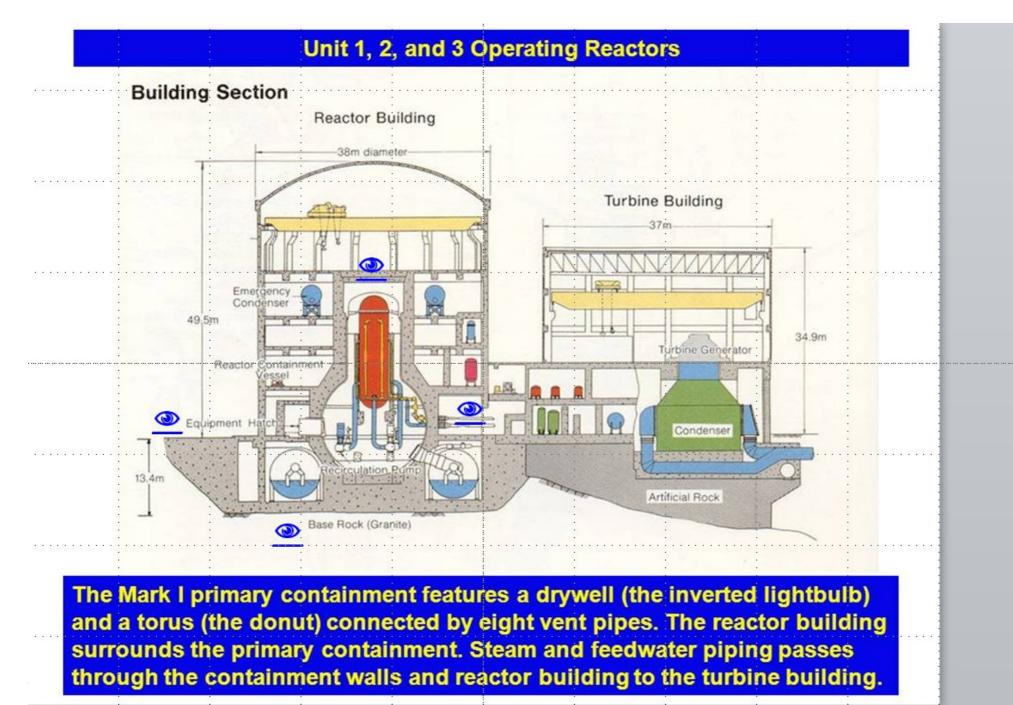
For the early boiling water reactors (BWR) of 1F with power outputs of 460 (1F1) or 784 (1F2-4) MWe (hence thermal power on the order of 1400 or 2400 MWt), electrically powered circulating pumps continued to cool the reactor pressure vessels and to reject the heat through heat exchangers to seawater. The reactors normally produced steam at about 950 psig (70 bar) and 540°F. Reactor 1F1 core comprised 69 tonnes of uranium in 400 fuel elements 435 cm long.
