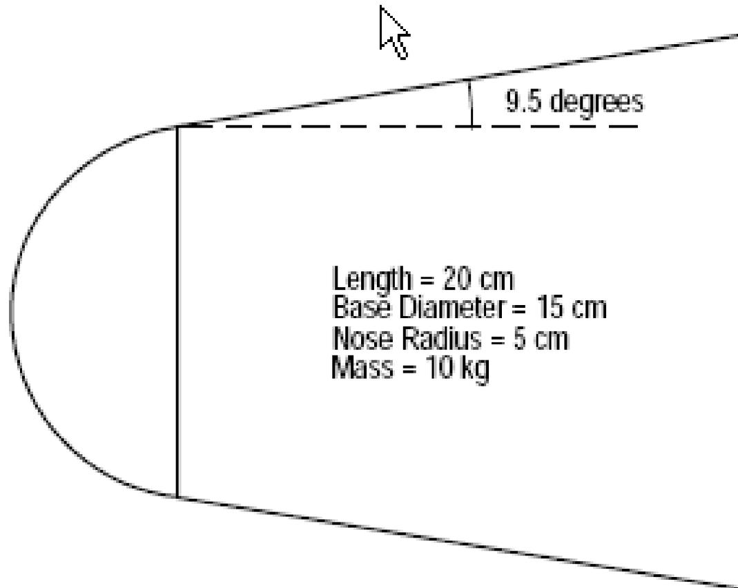
**Figure 7-1.** The configuration used for calculating the heating of a conical bomblet. *It has a nose radius of 5 cm, a base diameter of 15 cm, a length of 20 cm, a cone half-angle of 9.5 degrees, a mass of 10 kg, and a ballistic coefficient of 12,000 N/m<sup>2</sup> (250 lb/ft<sup>2</sup>).*
