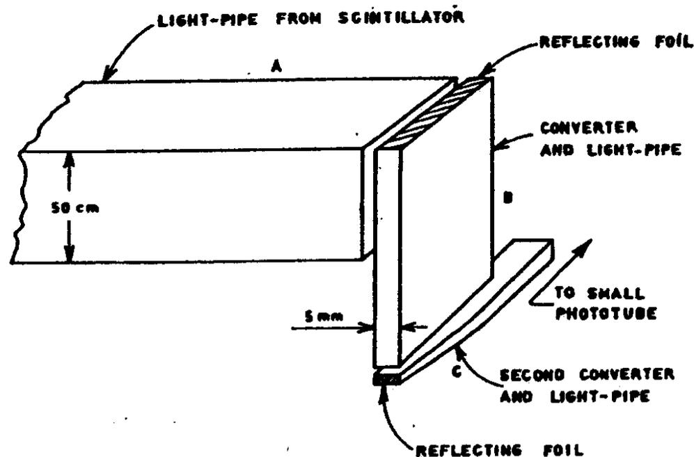
FIG. 1. Light from the light-pipe or scintillating vat (A) strikes converter (B), in which it produces fluorescent light of slightly lower photon energy. Some of this light, being isotropic, can now be collected along the converter without further loss; and, in principle, can be used a second time to produce fluorescence in the second converter (C) to concentrate further the light onto a small phototube.
